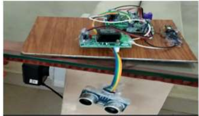
Figure 7.Obstacle sensor with IOT board
