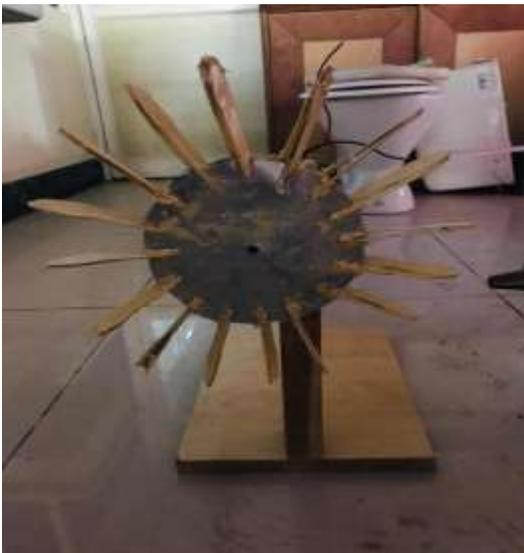
**Figure6 (a): model of turbine-wood**
