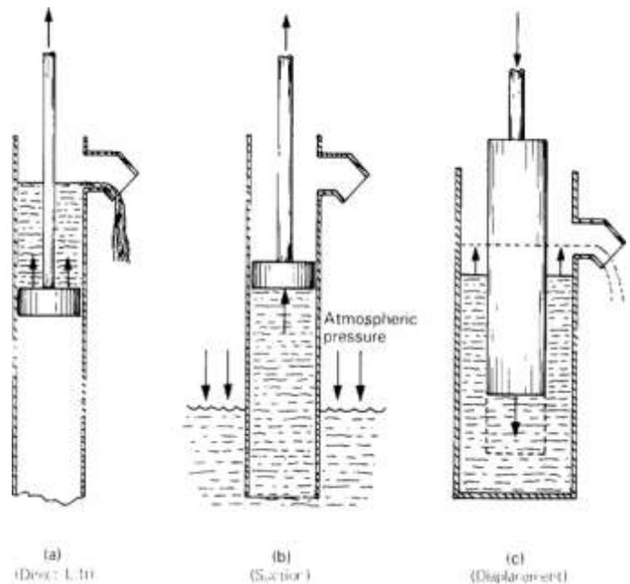
Figure5: Working of water piston pump
