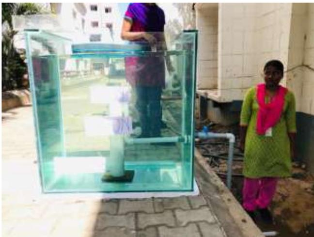
Figure 6(f): Wave flume and turbine setup
