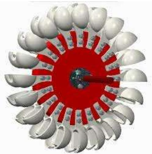
**Figure 6(c): Pelton wheel turbine**
