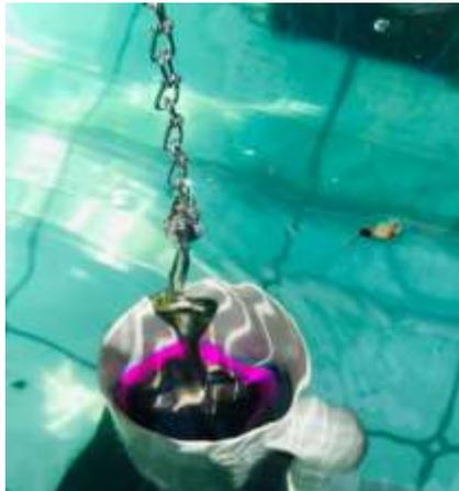
Figure 6(e): Buoy and piston connection in shaft
