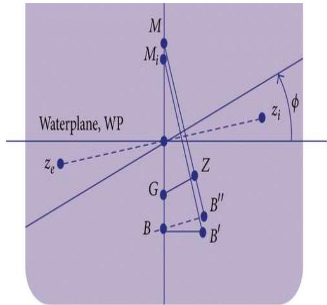
Figure 3: a floating device at an angle of inclination
