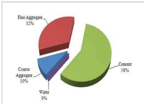
Figure 4. Cost contribution of each material to of OPC based concrete
