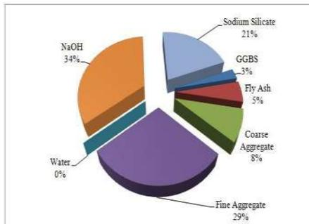
Figure 3. Cost contribution of each material to fly ash-GGBS based geopolymer concrete
