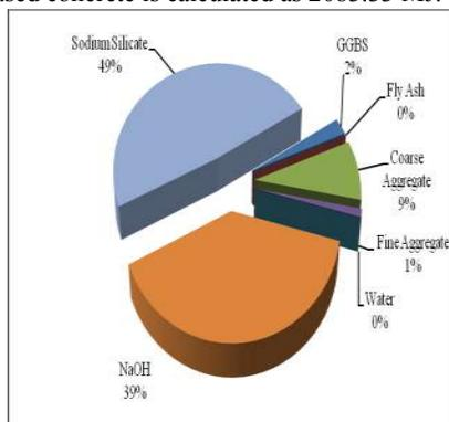
Figure 5. Embodied energy contribution of each material on fly ash-GGBS based geopolymer concrete.
