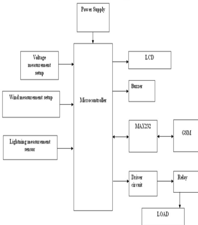
Figure 1: Block diagram of advanced power safety maintenance system
