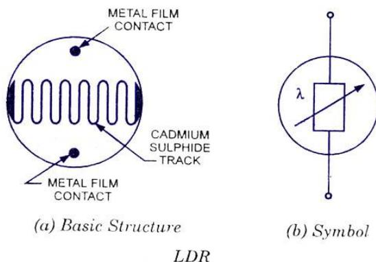
Figure 6: Basic structure and symbol of LDR
