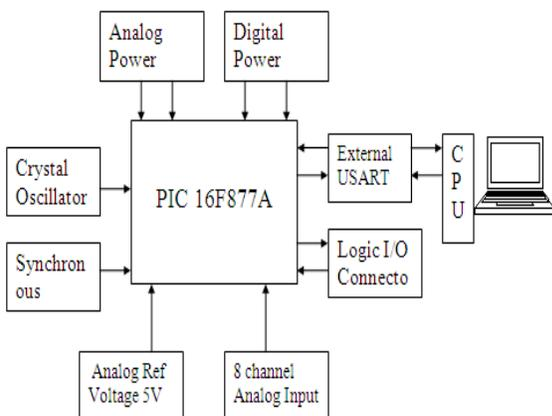
Figure 2: Block diagram of PIC
