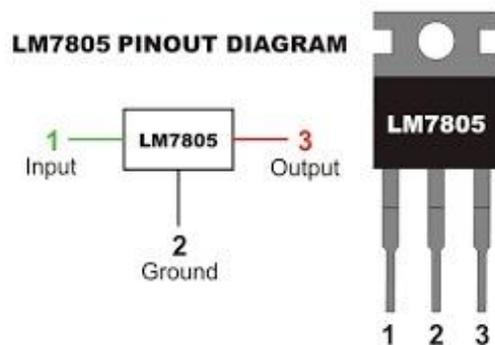
Figure 3: Pin diagram of regulator
