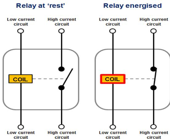
Figure 5: Circuit diagram of relay
