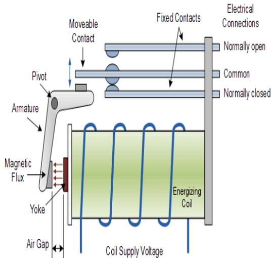
Figure 7: Schematic diagram of relay
