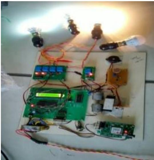
Figure12: Snapshot of on off control using GSM
