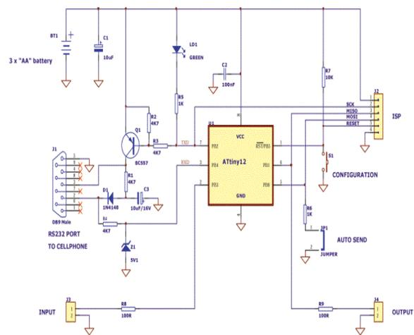
Figure 4: Circuit diagram of GSM
