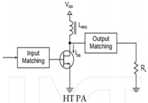
Fig.1 Class E inverter topology
