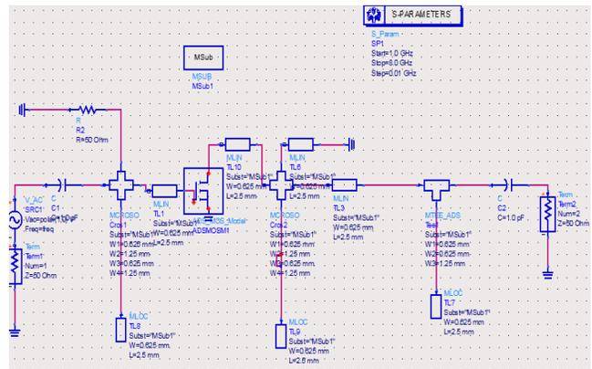
**Fig.5. Circuit schematic of transmission-line Class-E GaN HEMT power amplifier with shunt filter with capacitor**
