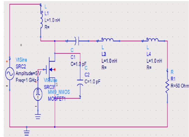
Fig.2. Class-E power Amplifier circuit
