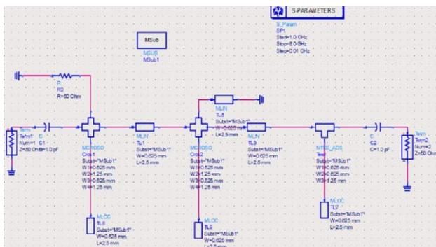
**Fig. 3.Circuit schematic of transmission-line Class-E GaN HEMT power amplifier with shunt filter with capacitor**
