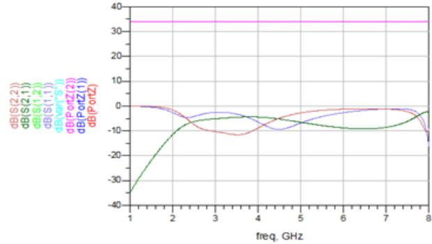
**Fig.4.Simulation result of transmission-line Class-E amplifier**
