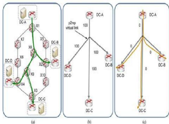
Fig.1 Light-tree-based VNT to serve an incoming multicast request
