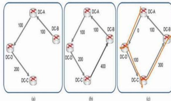
Fig.2 Multi-purpose VNT updating to serve an incoming multicast Request (a) Current virtual topology (b) Updated virtual topology (c) p2mp Provisioning
