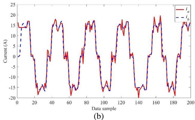
Fig. 8. A NOISE fault in the phase-A current signal: (a) original phase-A and phase-B current signals and (b) aligned current signals.
