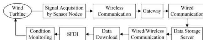
Fig. 1. Framework of a WSN-based wind turbine CMS.
