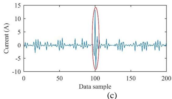
Fig. 4. Detection and isolation of a SHORT fault: (a) the corrupted stator phase current signal, (b) the approximation coefficients of the signal; and (c) the detail coefficients of the signal.
