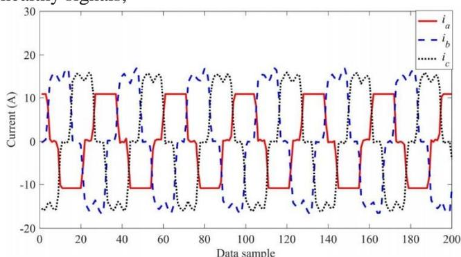
Fig. 6. Three-phase stator current signals with a CONSTANT fault in  $i_a$ .
