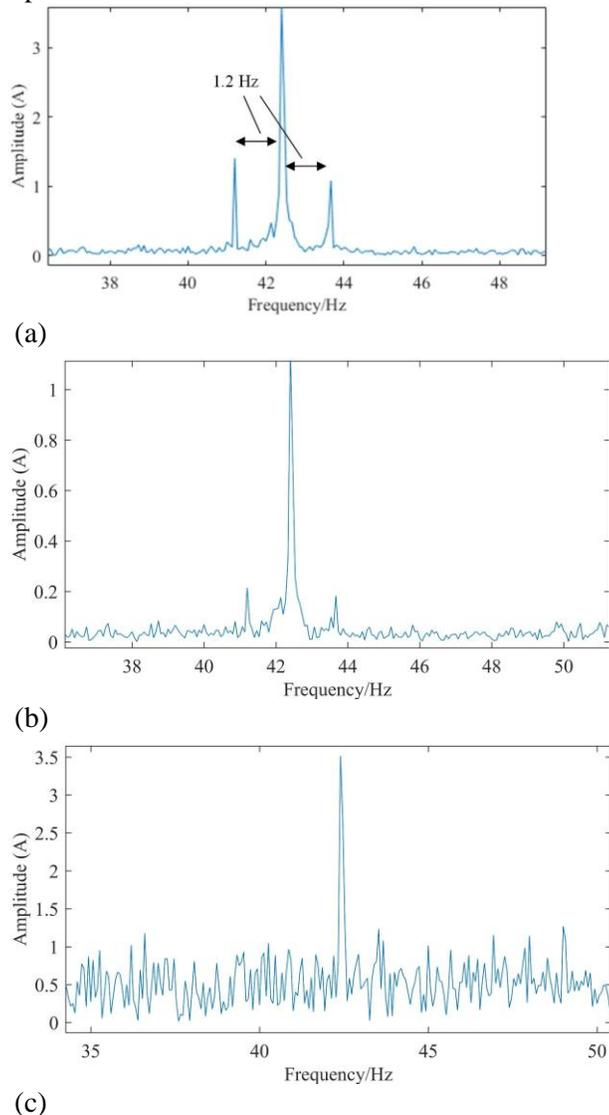
Fig. 10. Frequency spectrum of synchronously resampled current signal: (a) no sensor fault, (b) with a CONSTANT fault, and (c) with a NOISE fault.
