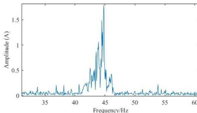
Fig. 9. Frequency spectrum of the original generator stator phase current signal around the fundamental frequency.
