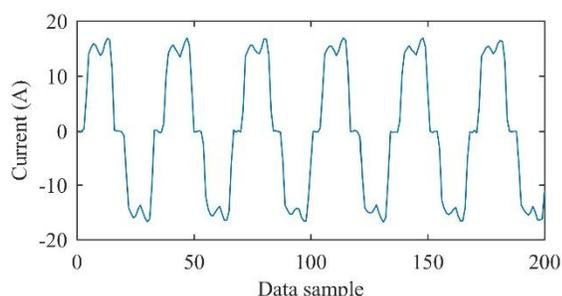
Fig. 5. Stator phase current signal after fault restoration. Since a CONSTANT fault causes a decrease in the cross-correlation between the faulty signal and the healthy signals,
