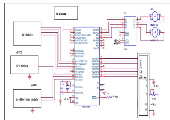
**Fig.5. Circuit of Soil Nutrient Monitoring**
