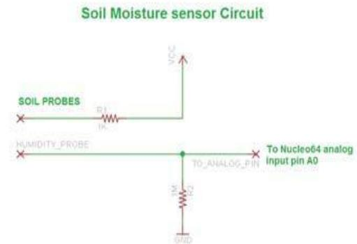
Fig. 3. Soil Moisture Sensor Circuit
