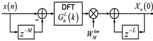
Figure 2. Modulated HDFT structure.
