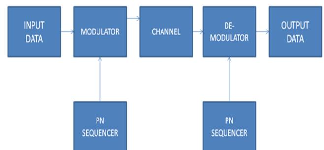
Fig.1 Basic model of DS-SS Communication System
