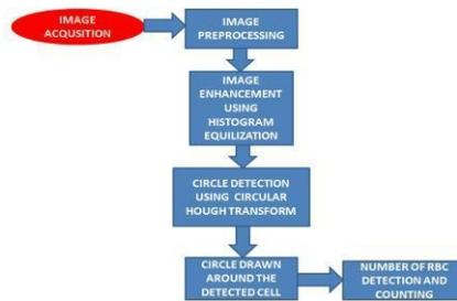
Fig. 4. Block diagram of RBCs detection and counting
