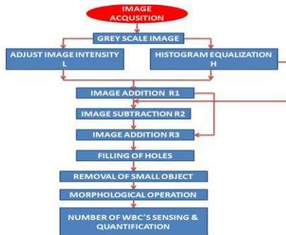
Fig.7. Block diagram of WBCs detection and counting
