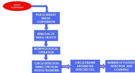
**Fig.9. Block diagram of Platelets detection and counting**
