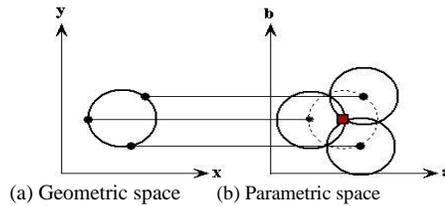
Fig.5. Each point in geometric space (left) generates a circle in parameter space (right).
