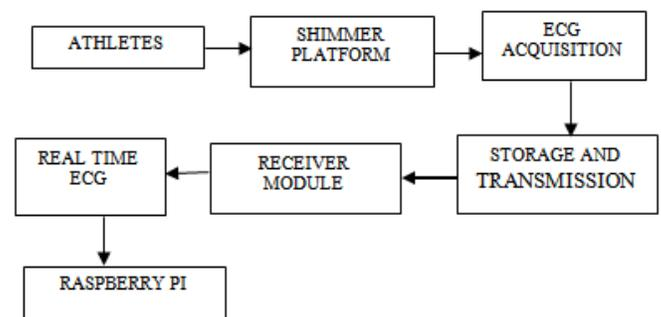
Figure 1. Block Diagram of the proposed model.
