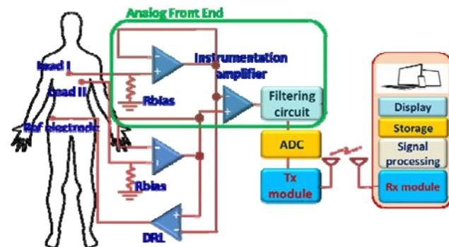
Fig. 2. General architecture of the ambulatory ECG monitoring system
