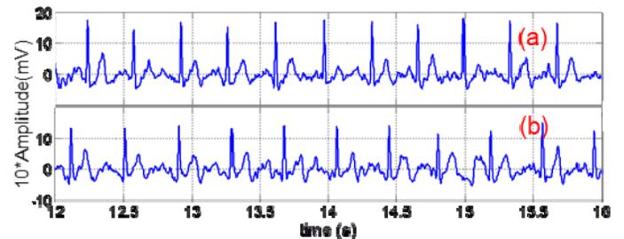
Fig. 7. ECG acquisitions in the time domain without body movement, with electrodes on (a) bare dry skin and (b) cotton fabric covered dry skin.
