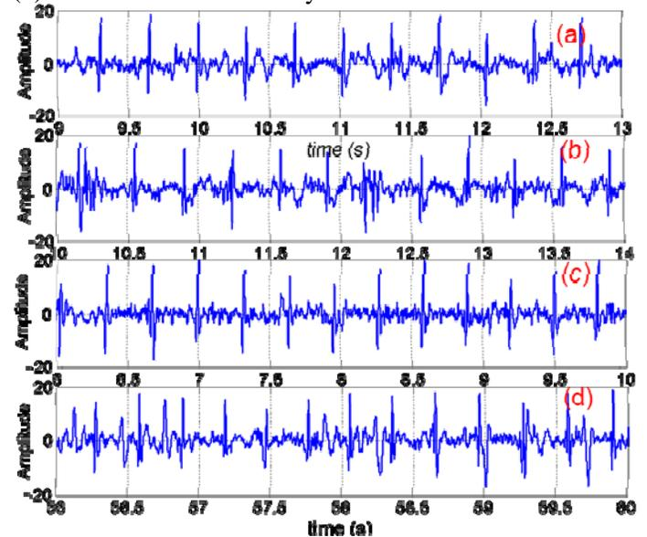
Fig. 8. ECG measured from the textile covered dry skin with body movements: (a) slow abduction-adduction of both hands, (b) fast abduction-adduction of both hands, (c) body rotation, and (d) normal walking.
