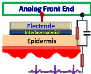
Fig. 4. Electrode-body interface with capacitive coupling of ECG bio-potential.
