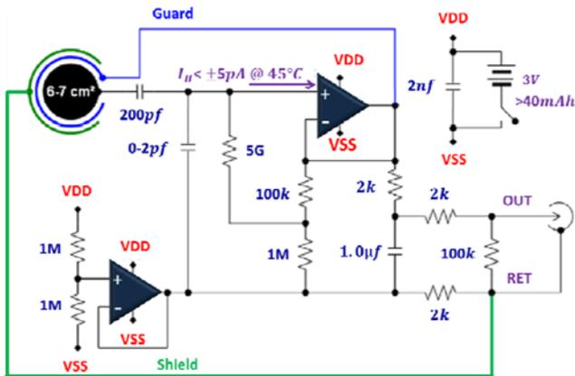
Fig. 5. Schematic diagram of the capacitive electrode.
