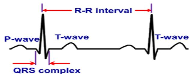
Fig. 1. Basic features in the waveform of an ECG signal
