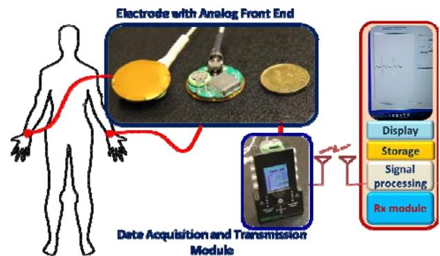
Fig. 3. Block diagram of the ECG sensing system with a photograph of a designed capacitive electrode.
