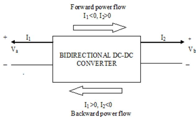
Fig.1. block diagram of bidirectional dc-dc converter
