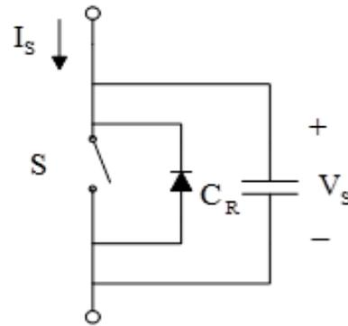
Fig.5. An Elementary resonant switch for achieving ZVS
