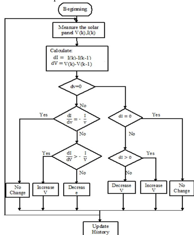
Fig.3. Flow Chart of Incremental Conductance Algorithm
