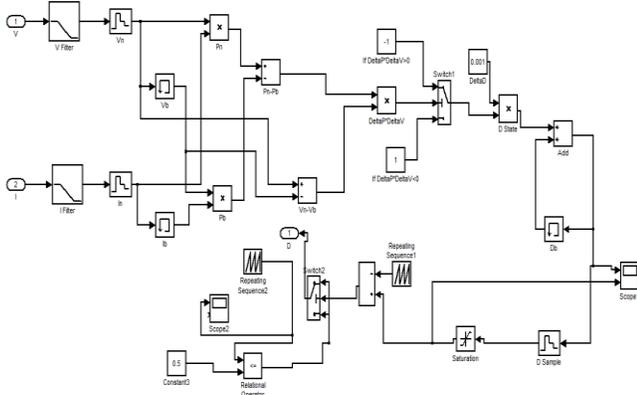
**Fig.8.Subsystems for Simulink Model of Incremental Conductance Algorithm**
