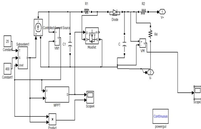
**Fig.7 subsystem of MPPT algorithm with boost converter**
