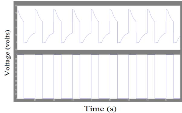
**Fig.11. ZVS of MOSFET Waveform**
