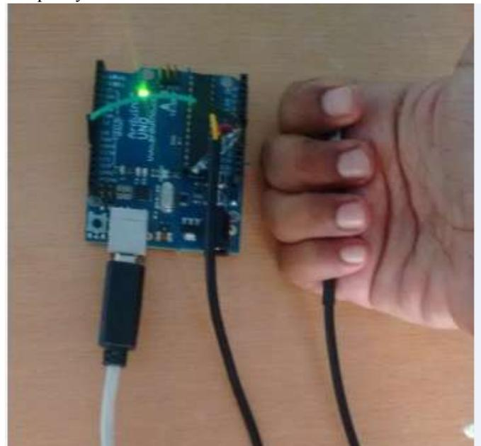
Figure 1 Hardware setup of Temperature sensor.
