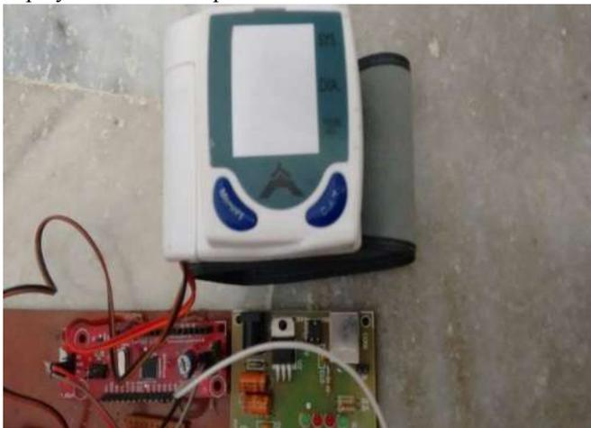
Figure 2 Hardware Setup of Blood Pressure Sensor
