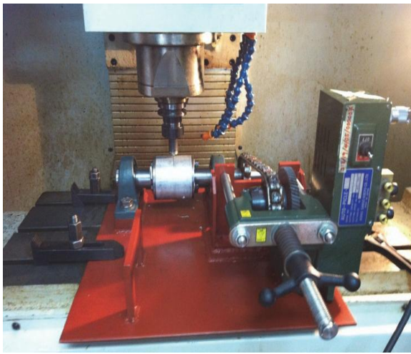
Fig.3: Orbital clamping unit for FSW experiment
