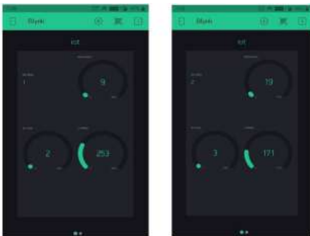
Fig. 7 IoT application displaying the fault at 1Km and 2Km distance
