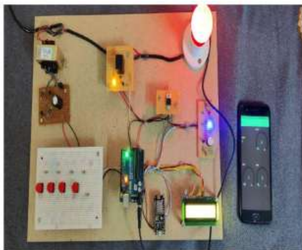
Fig. 2 Hardware model of IoT Based Underground Cable Fault Distance Detection System
