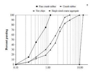
Fig.1. Gradation curve of aggregate, tire chips, crumb rubber, and fine crumb rubber
