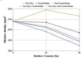
Fig.3. Fresh density of the pervious concretes versus rubber content
