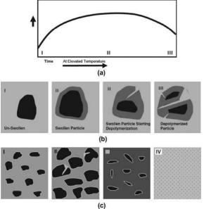
Fig.2. Progression of asphalt–rubber interaction at elevated temperature: (a) change in binder viscosity over time at elevated temperature, (b) change in particle size over time at elevated temperature, and (c) change in binder matrix over time at elevated temperature
