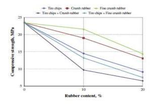
Fig.4. Compressive strength of pervious concretes versus rubber content
