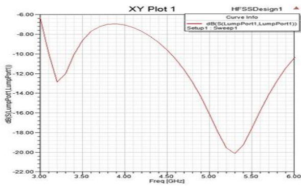
Figure 5.4 (a) Return loss plot for 2nd iteration of Koch Antenna
