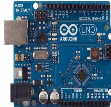
Fig 4.2 Arduino Uno Board
