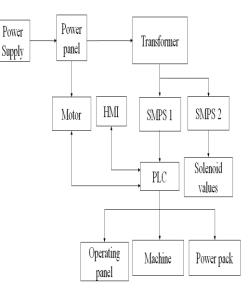
Figure 2.1 : Functional diagram
