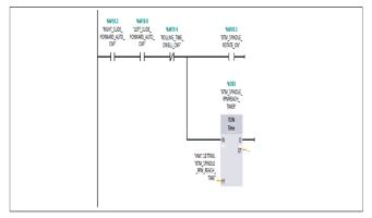
Figure 4.3 : Ladder logic for main ram up
