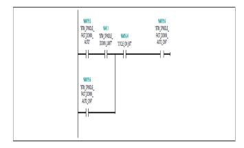
Figure 4.6 : Ladder logic for main ram down
