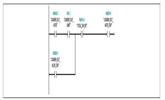
Figure 4.7 : Ladder logic for loader out confirm
