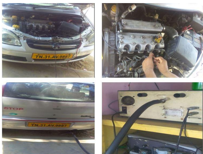
Fig.6.1.Emission Testing of Diesel Engine.
