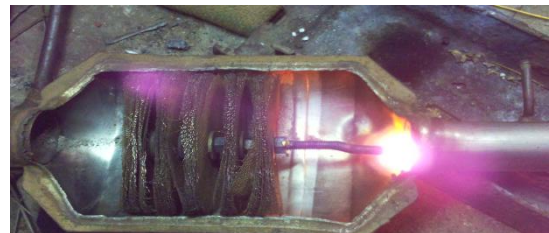
Fig.5.1.Welding of Catalyst substrate Package.
