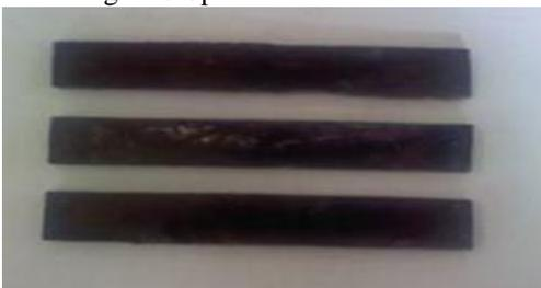
Figure.4.Specimen for flexural test
