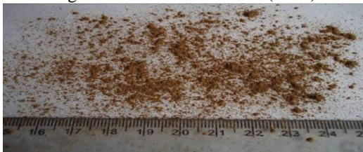
Fig.2. Coconut shell powder (CSP)
