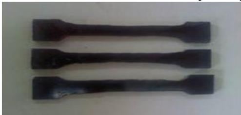
Figure.3.Specimen for tensile test
