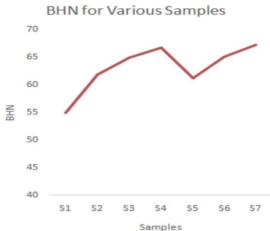
Fig 1. Effect of copper and magnesium content of Al-Cu-Mg Alloy
