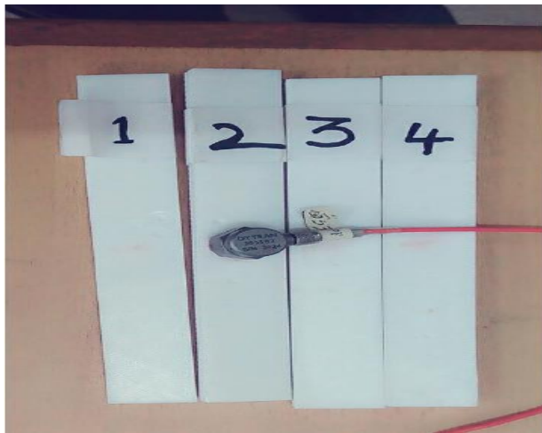
Fig 4 Rectangular Shaped ABS Specimens
