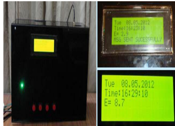
Fig.6:GSM Meter after casing and sample results on display.
