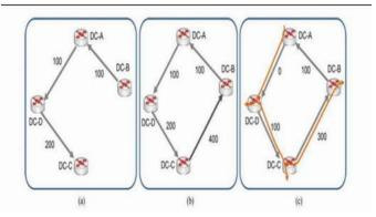
Fig.2 Multi-purpose VNT updating to serve an incoming multicast
