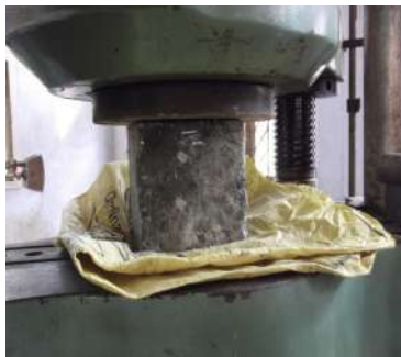
Fig 5 : Compression test on cube
