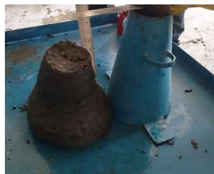
Slump Cone Test
