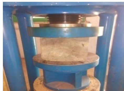
Figure 3 compressive test on cube
