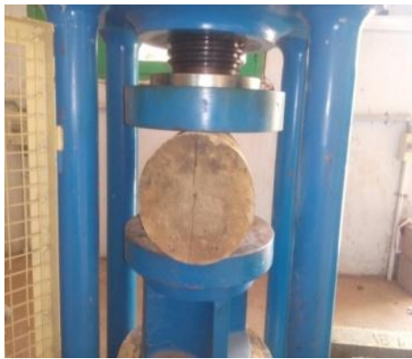
Figure 4 split tensile test on cylinder
