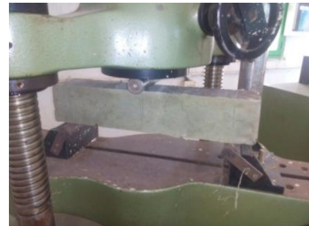
Figure 5 flexural test on prism
