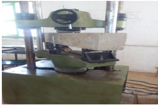
Figure 6 deflection test on beam
