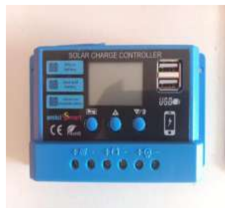
Figure 10 : PWM charging controller
