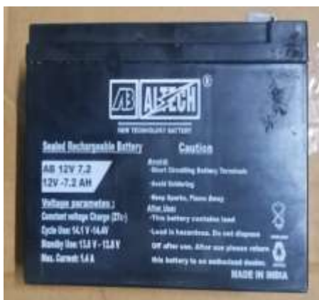
Figure 12 : Lead Acid Battery
