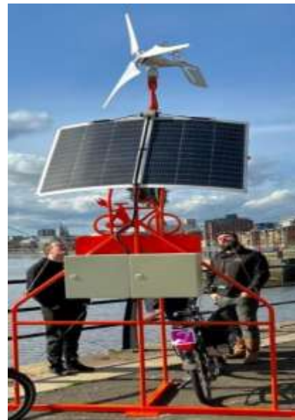
Figure 4 : Hybrid powered E-cycle charging station
