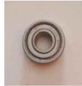
Figure 15 : The rolling element Bearing
