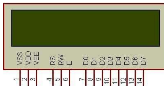
Figure 8 :LCD PIN DIAGRAM
