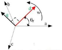
Figure.5. Park transform for AFPMSG generators.
