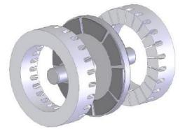
Figure.2.Magnetic circuit parts of an AFPMSG with one rotor-two-stators.
