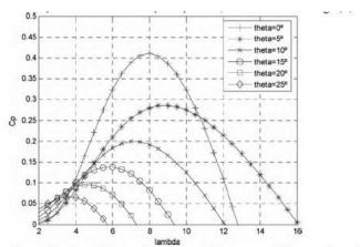
Figure.3. Coefficient of power (Cp) versus Tip-speed ratio (lambda)
