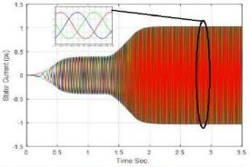
Figure.16. Three-phase stator currents in p.u
