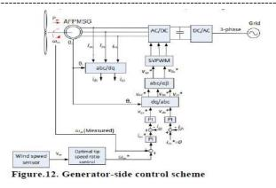
To collect the comments present day alerts, 3segment stator currents are sensed and transformed into the dq-axes reference frame in line with Park's transformation. The reference stator voltages are then being done through PI controllers in the dq-axes contemporary control loops. here, the space vector pulse width modulation (SVPWM) method is carried out as the modulation strategy in this machine, as it generates much less harmonic distortion inside the output stator voltages/currents and offers
