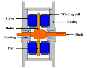
Figure.1. Cross section views of the AFPMSG
