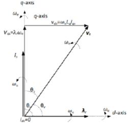
Figure.11. Phasor diagram of the FOC
