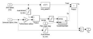
Figure.4. Wind turbine Simulink model.
