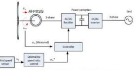
Figure.10. Tip speed ratio control scheme
