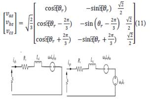
Figure.6. The *dq*-axes equivalent circuits of a AFPMSG in (consumer/load) notation
