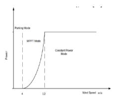
Figure.9. Wind turbine power-speed characteristic for the specific wind turbine
