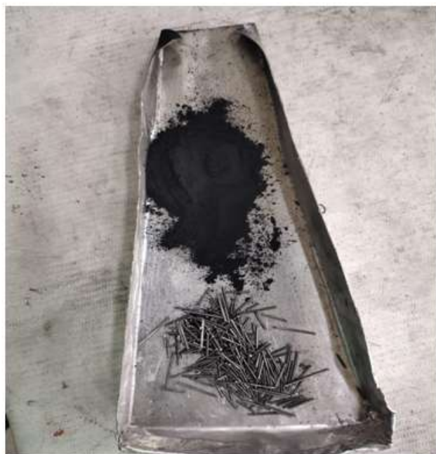
Fig-5 grapheme and steel wires
