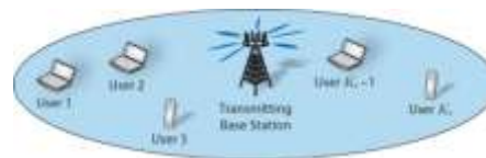
Figure 1.3 Illustration of the downlink multi-user system in Section 1.2. A base station with N antennas serves K_r users.
