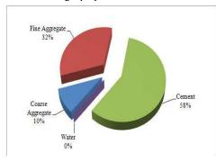
Figure 4. Cost contribution of each material to of OPC based concrete Studies have to be made in the area of manufacturing process of sodium hydroxide so as to make its cost less. The fine aggregate cost can be minimized by using alternate materials like crusher dust. However, the impact of using such materials on the strength of concrete has to be studied.
