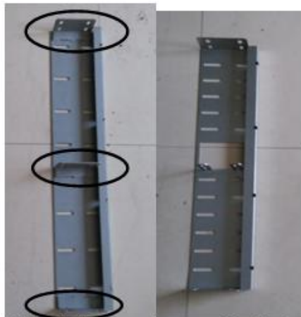
Existing Design New Design ➤ Material: Existing – 2 mm GI New – 2mm GI ➤ The Welding & Painting process eliminated from the existing design
