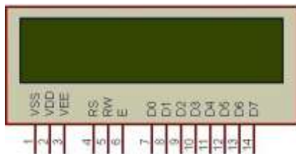
Figure 11 : LCD Pin diagram (16*2)
