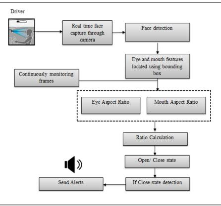
driver's state. The CNN architecture may include convolutional layers followed by fully connected layers for classification. Upon detecting drowsiness, the system triggers alerts, such as visual warnings or automated actions, to prevent accidents. Continuous monitoring ensures real-time responsiveness. The system can be integrated into vehicles for proactive safety measures, enhancing road safety by mitigating the risks associated with driver drowsiness.
