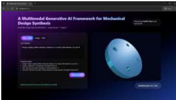
Fig. 1 Text-to-CAD generation module demonstrating automated flange coupling model creation.
