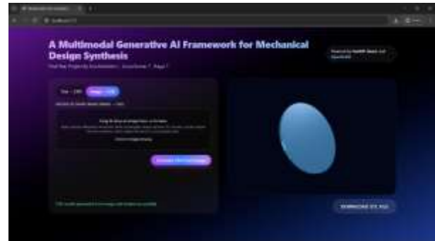
Fig. 3 Circle silhouette converted into a solid 3D model using the image-to-CAD module.
