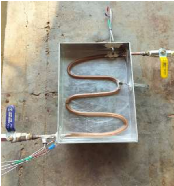
Fig. 2 Fabricated Experimental Setup for PCM Based Thermal Management System
