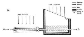
Fig. 10. Single slope solar still assimilated to tubular solar collector [19] Singh et al. [19] theoretically analyzed the performance of a solar still assimilated to evacuated tube collectors. Parameters such as number of collectors, water depth were optimized for higher efficiency and yield from the solar still. The results showed that the energy and energy efficiency was higher inthe case water depth (dept of
