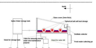
Fig. 3. Schematic diagram of a conventional solar still with sphericalball (Encapsulated) salt heatstorage
