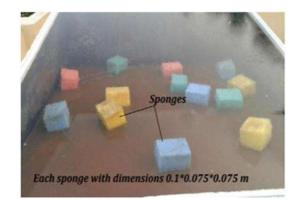
(b) Experimental photograph of a conventional solar still withsponges Fig. 4. Experimental setup
