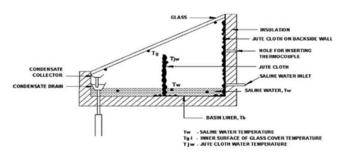
Fig. 6. Schematic diagram of a single slope solar still with vertical jute cloth
