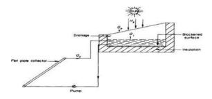
Fig. 9. Single slope solar still coupled to flat plate collector [18]
