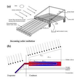
Fig. 11. Schematic diagram of (a) Evacuated tube collectors assimilated to conventional solar still [20] (b) Thermo syphon operation mode in evacuated
