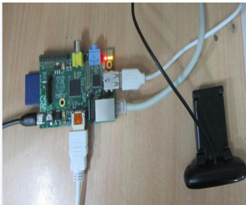
Fig 2: Connection Of USB Camera With Raspberry Pi
